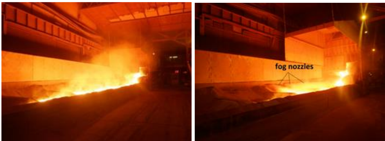
Figure 6: HCFeMn casting bed without (left) and with fog nozzles in operation (right)
