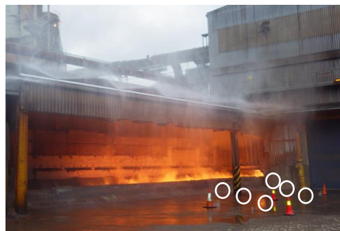
Figure 2: Catch pots set up around the casting beds to capture water samples Cowx et al. (2015)
