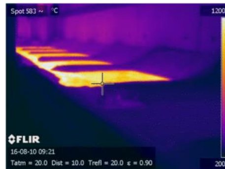
Figure 1: IR photograph of the casting beds Gates et al. (in press)
